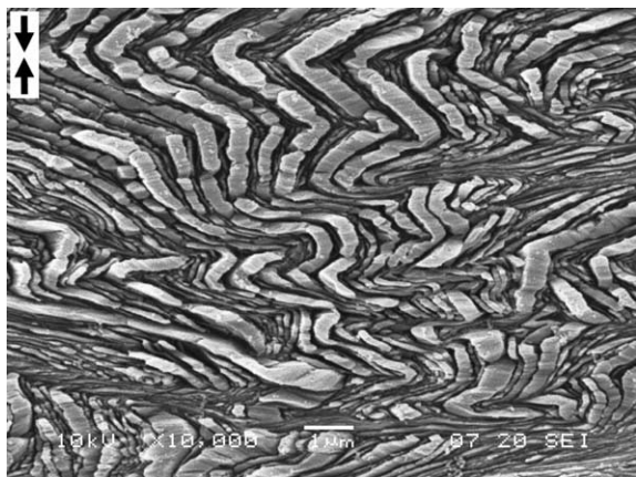
Fig. 8. Scanning electron micrographs of etched surface exposed by sectioning of high density polyethylene samples having 156 nm thick crystals and 87% of crystallinity subjected to compression with the ratio of 3.175. No lamellae fragmentation is observed at such compression ratio.
